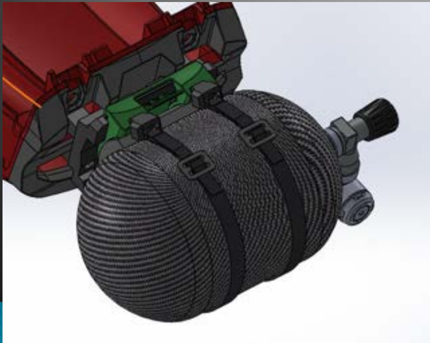
Custom oxygen tank locator for military mine sweeping diving equipment and strap assembly method
