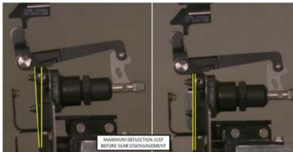
Flex in bracket before and after stiffening bracket modification
